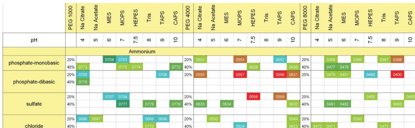
Figure 3 A chemical space map with the cells colored according to the crystallization result. The red color indicates a crystal hit, light green a precipitate, dark green a skin and turquoise a clear result. Multiple category results are shown by cross-hatched colors, with each color representing one of the categories. In this illustration, the blocks which appear orange are cross-hatched with alternating red and light green to indicate a combination of crystals and precipitate.
